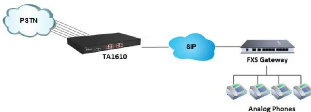
Figure 2-3 Connect TA FXO Gateway and FXS Gateway
